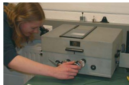
Verification by means of the interference comparator at the KOBA laboratory.
